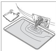
4. When the container is full of water, put the drainage duct back again and empty the container. Repeat step 3 until no more water flows out from the drain pump.
