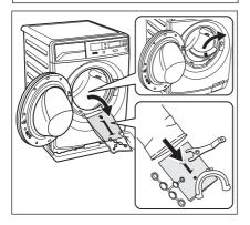
Open the door. Remove the polystyrene piece from the door seal and all the items from the drum.
