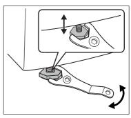
When the washing machine is levelled, try to rock it from corner to corner. If it does rock, adjust the legs again until it is levelled and does not rock.
