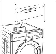
If you do not have a spirit level, as a guide use the edge of a door frame, cupboard or bench to check that the washing machine is level.
