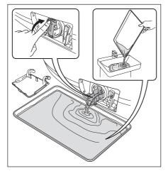
5. Pull back the drainage duct and turn the filter anti-clockwise to remove it.
