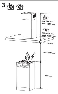
**Note**: Some installations may require the telescopic exhaust cover to be cut to lenght. Cut with sharp tin snips or a fine-tooth hack saw blade, taking care not to distort or dent the exhaust cover.
