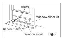
Cut the adjustable window slider kit if the width of window is less than 67.5cm (Fig. 10).
