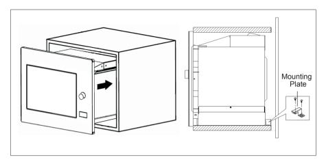
2. Open the door and fix the oven to the cabinet with Screw B, at the installation hole. Then fix the Trim-kit plastic cover to the installation hole.
