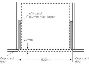
Infill panels are recessed 20mm from the external cabinet door to accommodate flush fit.
