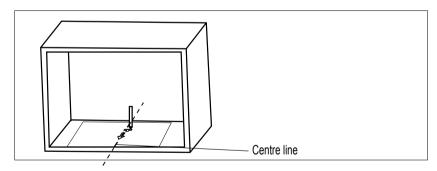
3. Remove the bottom cabinet template and fix the mounting plate with screw  ${\sf A}.$
