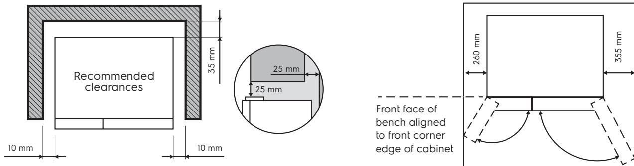
When positioned in a corner area, spacing of right side at least 260 mm and left side at least 355 mm on the hinge side will allow the doors to open enough to enable the removal of bins and shelves.
